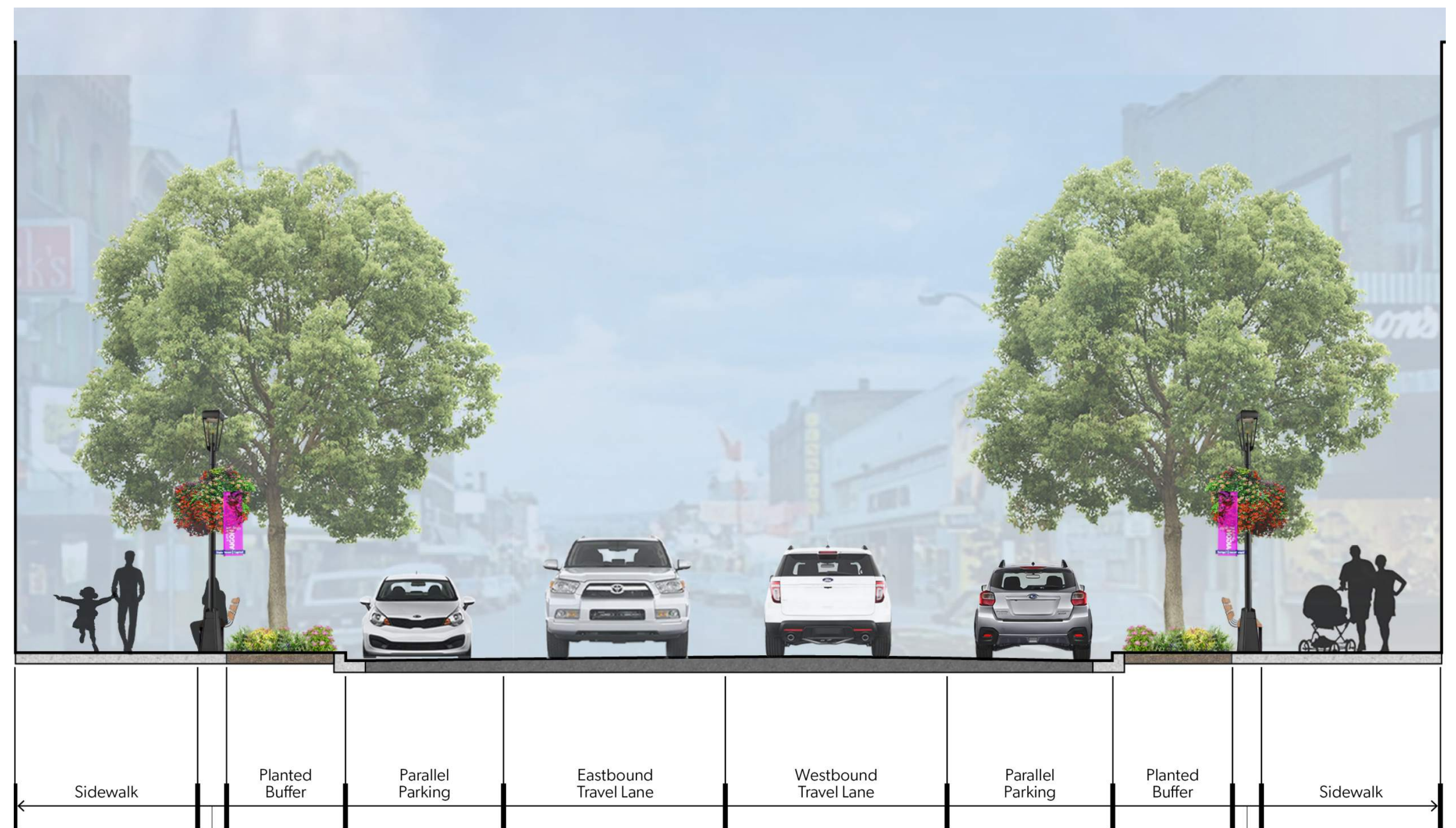
The typical section on Main Street, including two-way traffic, was determined through a previous study.
