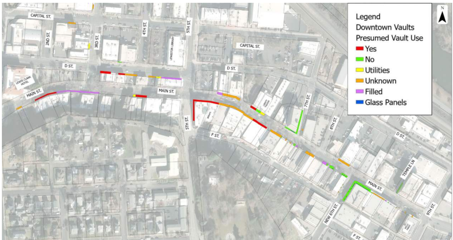
Current status of known sidewalk vaults in the project area.
