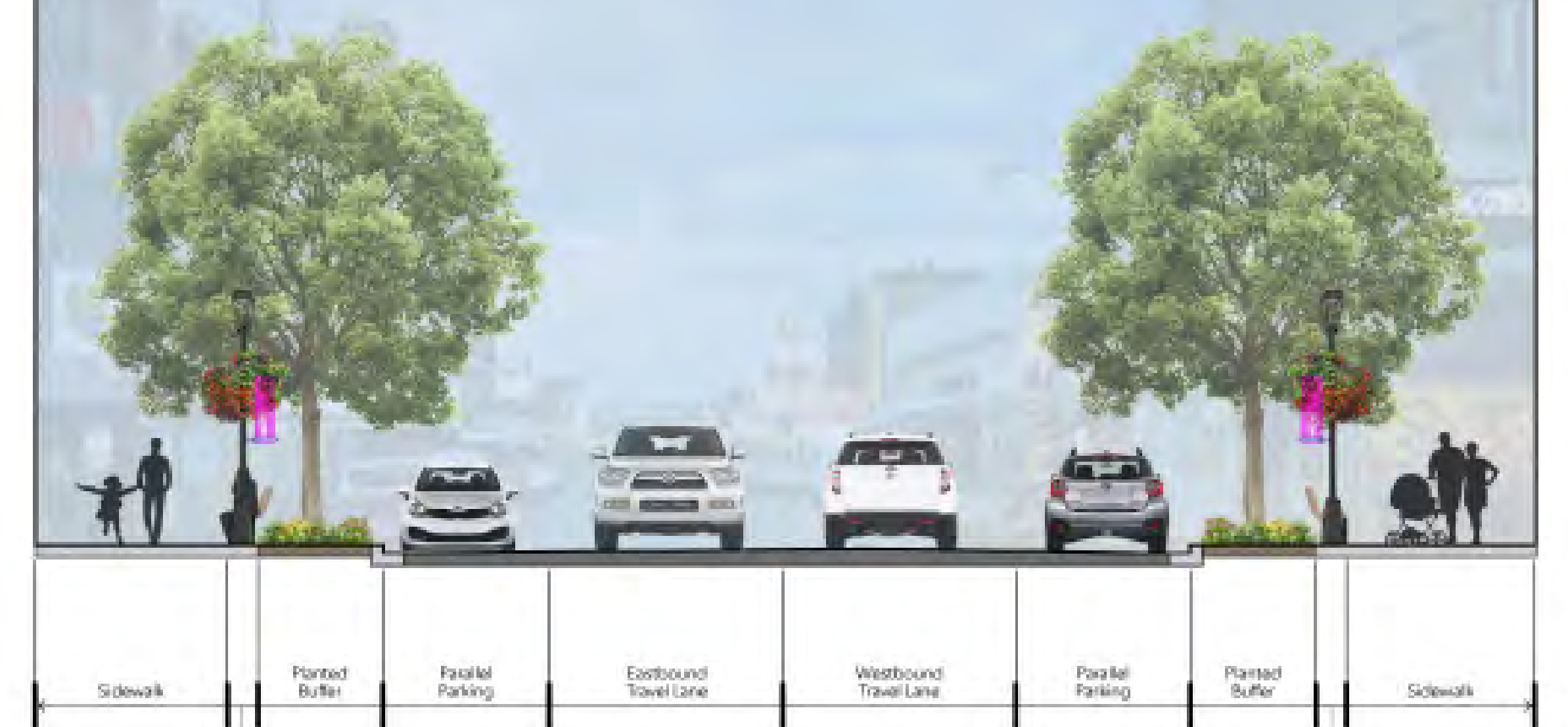
The typical section on Main Street, including two-way traffic, was determined through a previous study.
