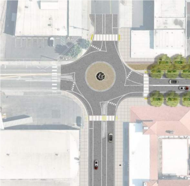
1 st Street/D Street Stop Compact Roundabout Concept
