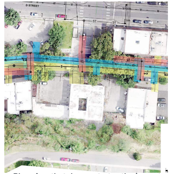
Plan view that demonstrates the impact aboveground when replacing underground infrastructure.
